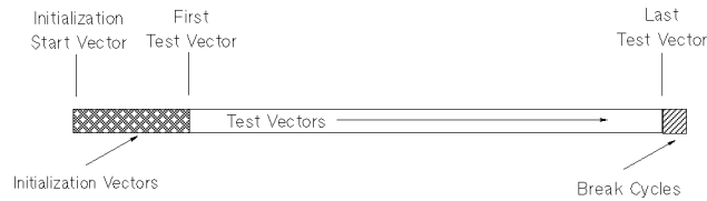
Figure 6-14. Executing a Single Block of Vectors with an Initialization Block
